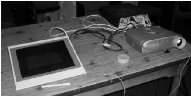
Fig. 1. Lectern II setup as seen by instructor. Setup consists of touch-sensitive screen, digital pen, microphone, PC, and a video projector.
